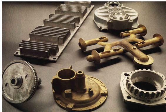
**Figure 1.** Application of ZA-27 alloy
