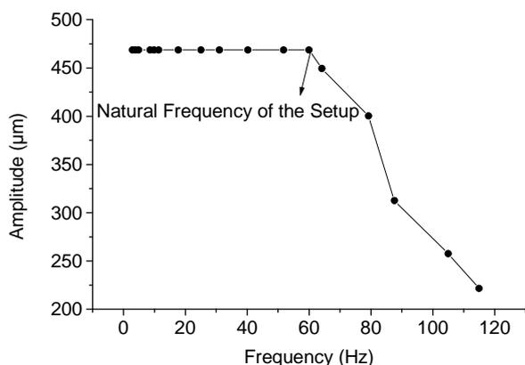
**Figure 2.** Amplitude vs. frequency curve of the test setup for without added dead load
