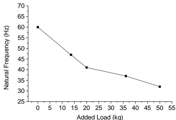
**Figure 4.** Variation of natural frequency with the variation of dead added loads
