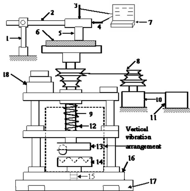
**Figure 1.** Schematic diagram of the experimental setup: 1. Load arm holder 2. Load arm 3. Normal load (dead weight) 4. Horizontal load 5. Pin sample 6. Test disc with rotating table 7. Computer 8. Belt and pulley 9. Main shaft 10. Motor 11. Speed control unit 12. Compression spring 13. Upper plate with ball 14. Lower plate with V-slots 15. Height adjustable screw 16. Base plate 17. Rubber block 18. Added dead load
