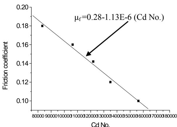
**Figure 8.** Friction coefficient as a function of chowdhury no.
