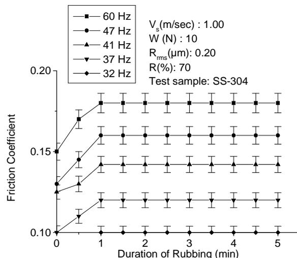
**Figure 5.** Variation of friction coefficient with the variation of natural frequency of the experimental setup
