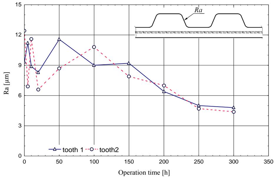
**Figure 9.** Change of  $R_a$  at the flank of the belt's tooth during operation
