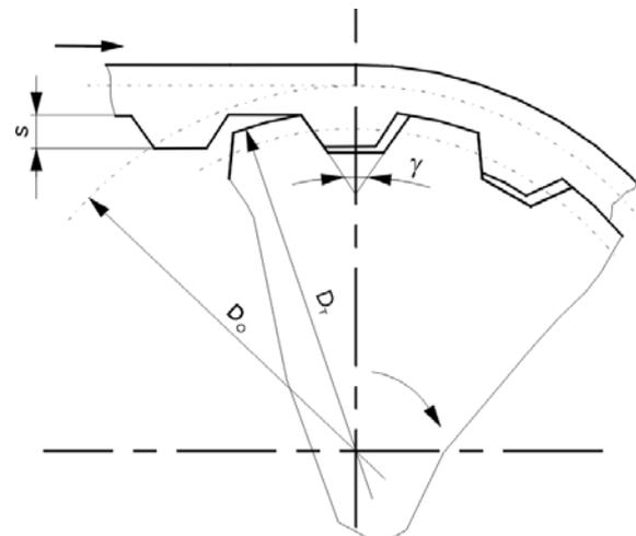
**Figure 1.** Layout of coupling between the belt and the drive belt pulley
