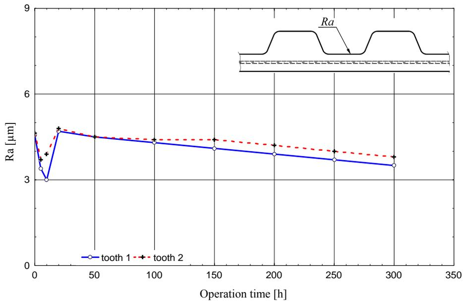
**Figure 11.** Change of  $R_a$  at the space between belt's teeth during operation
