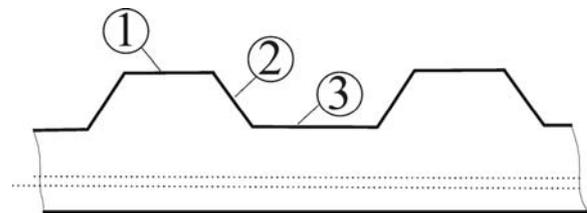
**Figure 4.** Measuring points on the belt for measurement of roughness parameters
