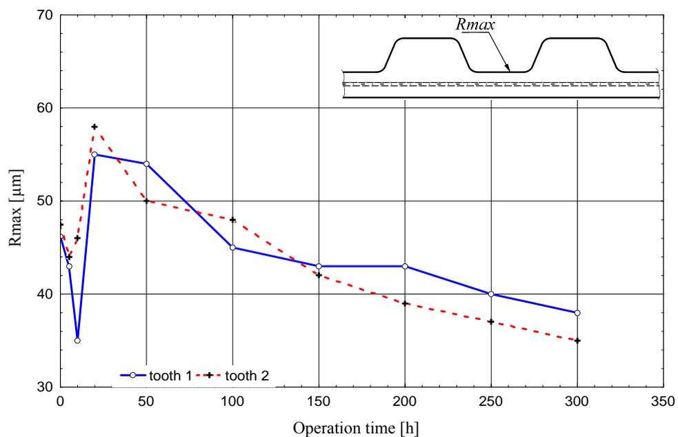
**Figure 10.** Change of  $R_{max}$  at the space between belt's teeth during operation
