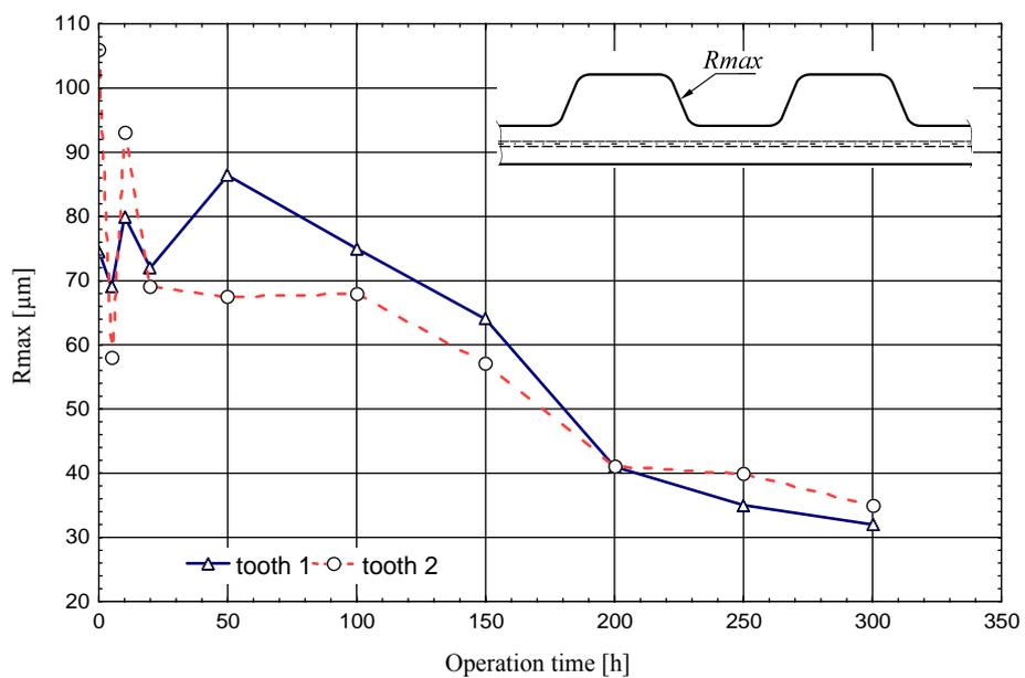
**Figure 8.** Change of  $R_{max}$  at the flank of the belt's tooth during operation
