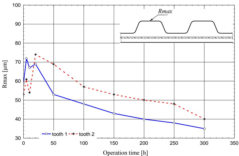
**Figure 6.** Change  $R_{max}$  at the apex of the belt's tooth during operation
