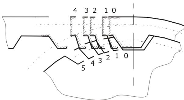
**Figure 2.** Layout of belt's teeth entering the coupling with the teeth of the drive belt pulley
