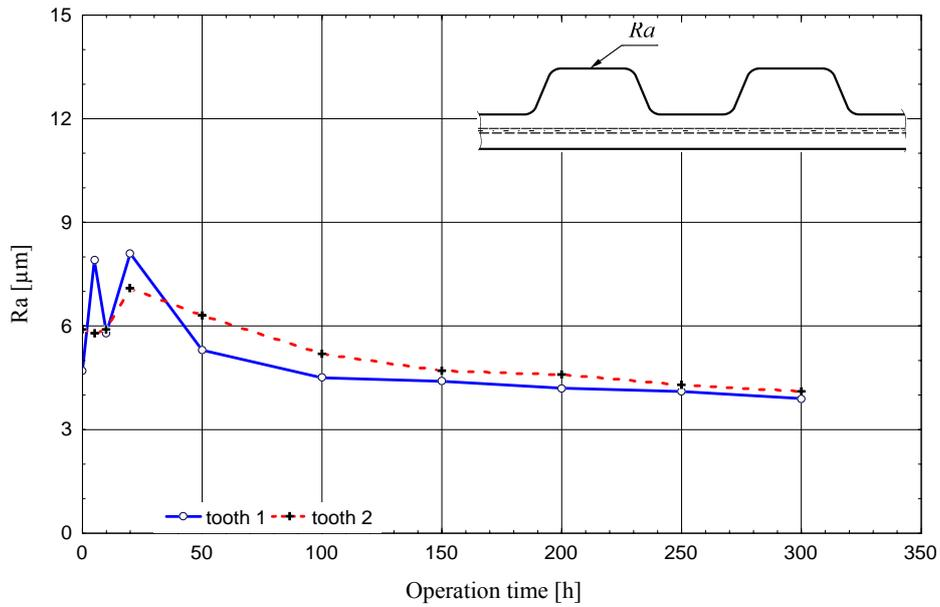
**Figure 7.** Change  $R_a$  at the apex of the belt's tooth during operation
