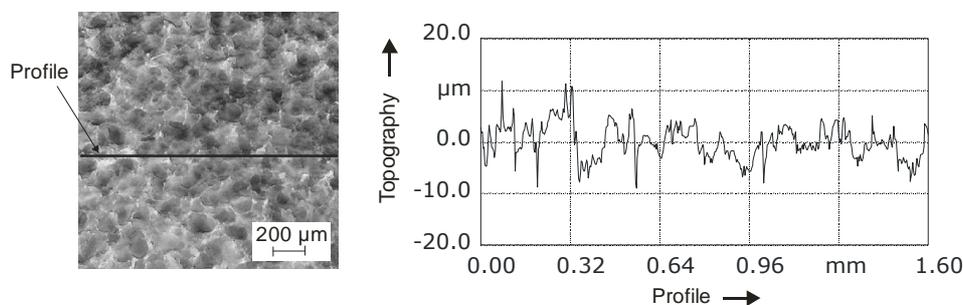
**Fig. 3.** Topography generated by pre-finishing (EDM).
