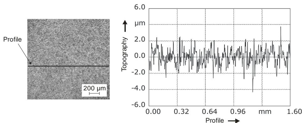
**Fig. 4.** Topography generated by finishing (EDM).
