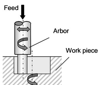
Fig. 2. Principle of polishing process.
