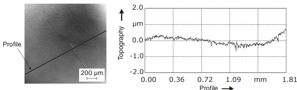
**Fig. 11.** Topography of polished surface hard machined by pre-finishing (EDM).
