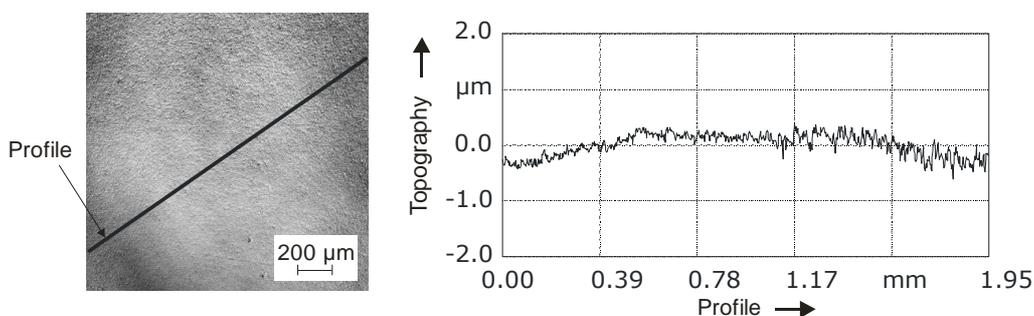
**Fig. 12.** Topography of polished surface hard machined by finishing (EDM).
