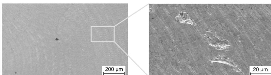
**Fig. 9.** Topography and surface defects generated by pre-finishing (grinding).
