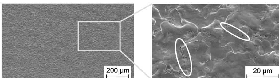
**Fig. 6.** Topography and micro-cracks generated by finishing (EDM).
