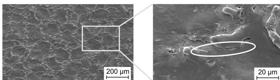
**Fig. 5.** Topography and micro-cracks generated by pre-finishing (EDM).
