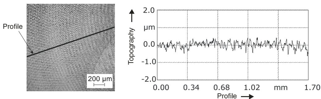
**Fig. 7.** Topography generated by pre-finishing (grinding).
