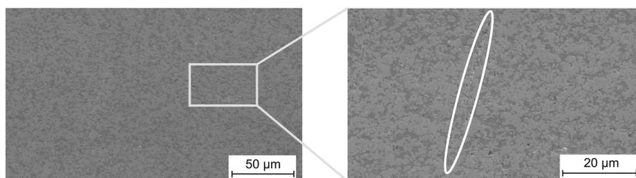
**Fig. 13.** Topography of polished surface hard machined by pre-finishing (EDM).
