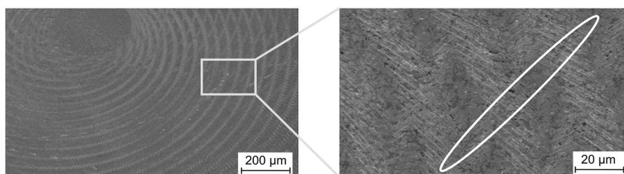
**Fig. 10.** Topography and surface defects generated by finishing (grinding).
