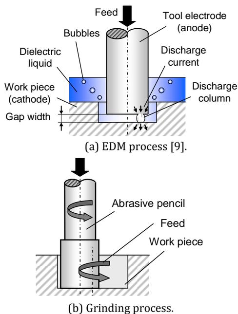
**Fig. 1.** Characteristics of hard machining methods.
