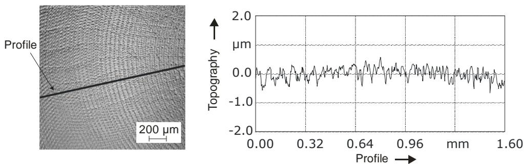
**Fig. 8.** Topography generated by finishing (grinding).
