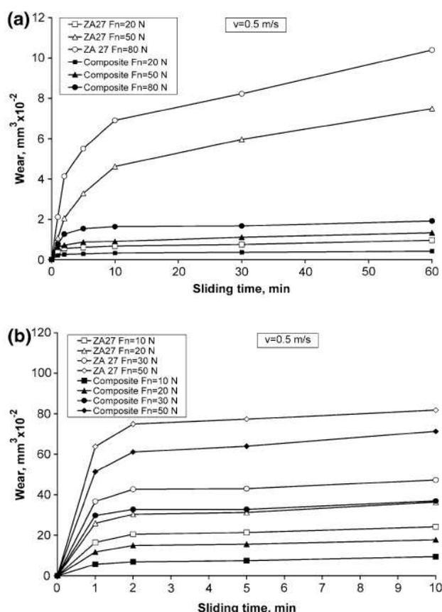
Fig. 1. Wear curves of tested materials; a) Lubricated sliding, b) Dry sliding [2,4].
