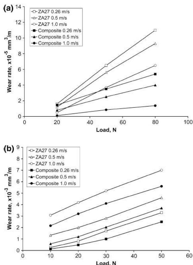
Fig. 2. Wear volume vs. applied load; a) Lubricated sliding, b) Dry sliding [2,4].
