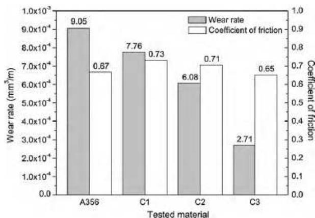
**Fig. 14.** Wear rate and coefficient of friction values of heat treated (T6) A356 aluminium alloy, composite C1 (with 10 wt% Al<sub>2</sub>O<sub>3</sub> particles), composite C2 (with 10 wt% SiC particles), and composite C3 (with 10 wt% SiC and 1 wt% graphite particles) [32,33].
