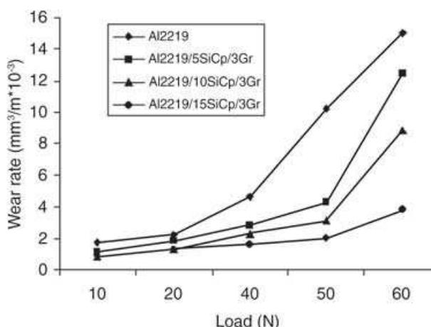
Fig. 9. Variation of wear rate with applied load at a sliding speed of 3 m/s for a sliding distance of 5000 m [20-22].
