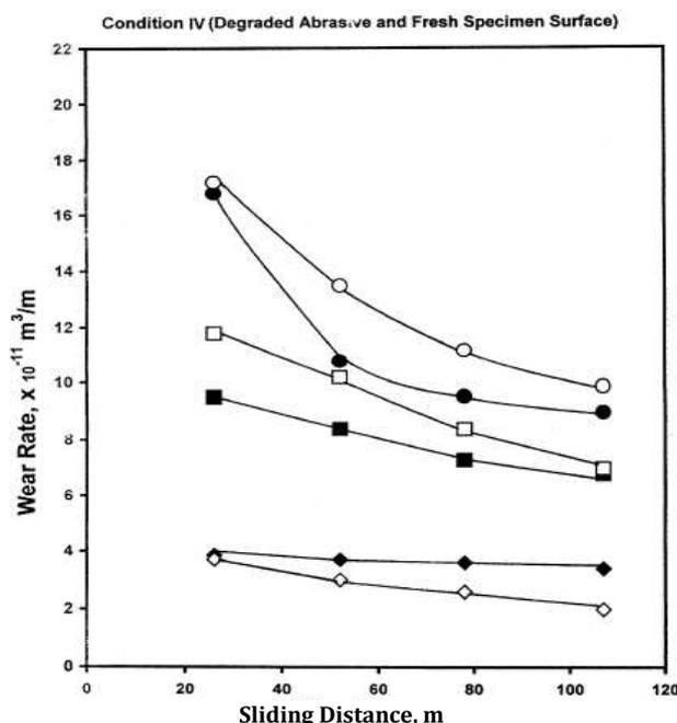
**Fig. 5.** Wear rate of the specimens as a function of sliding distance at various applied loads in experimental condition (open symbols: composite; closed symbols: matrix alloy,  $\blacklozenge$ : 1 N,  $\blacksquare$ : 3 N,  $\blacktriangle$ : 5 N,  $\bullet$ : 7 N [13]).
