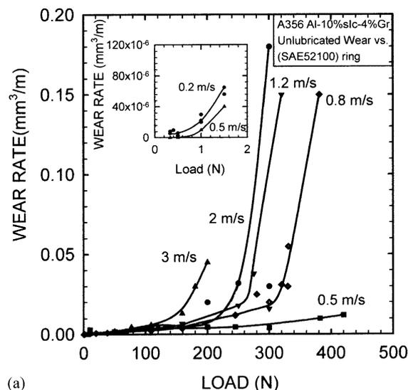
Fig. 11. Wear volume vs. applied load [26].
