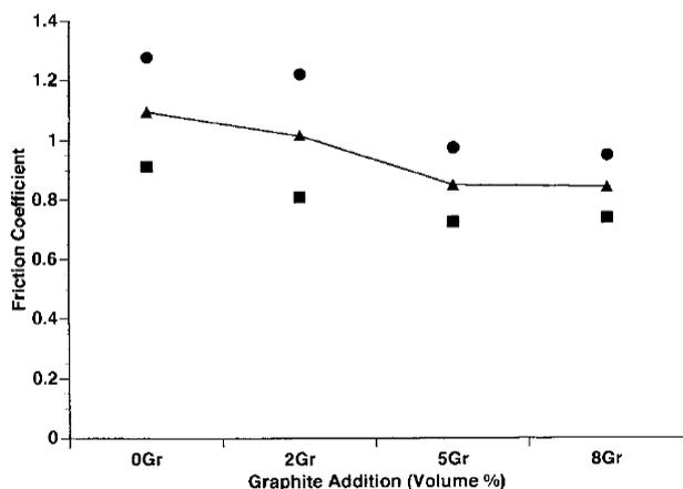
Fig. 6. Variations of friction coefficient with the percentage of graphite addition [19].
