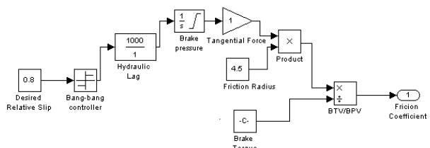
**Fig. 12.** Simulink model for single wheel disc brake.
