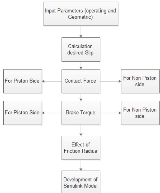
**Fig. 10.** Algorithm for friction coefficient estimation.
