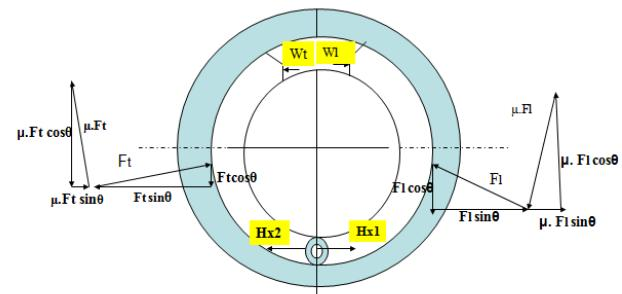
**Fig. 3** Force analysis for both the shoes of the drum brake.
