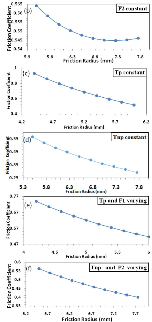
**Fig 18 (a-f)** Friction coefficient profiles for variations in friction radius for disc brake.
