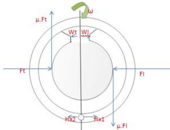
**Fig. 1.** Equilibrium diagram for the drum brake when contact force is normal.
