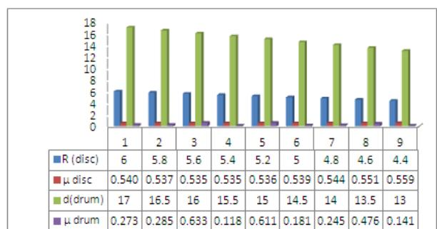
**Fig. 19.** Comparison of friction coefficient ( $\mu$ ) with friction radius.
