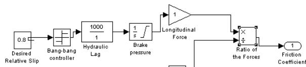
**Fig. 11.** Simulink model for single wheel drum brake.
