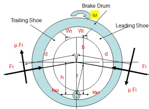
**Fig. 2.** Equilibrium diagram for the drum brake when contact force is inclined.
