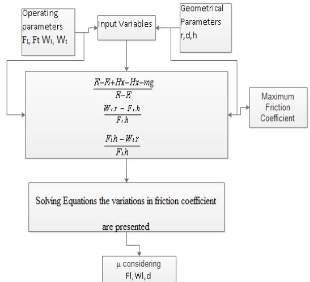
**Fig. 9.** The flowchart for friction coefficient estimation.
