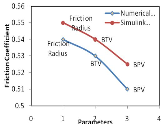
**Fig. 14.** Comparison of output for numerical and simulink based estimation.
