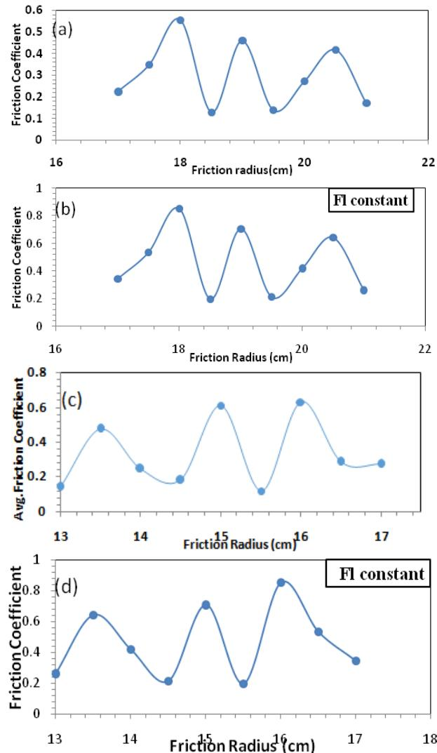
**Fig. 17 (a-d)** Friction coefficient profiles for variations in friction radius for drum brake.
