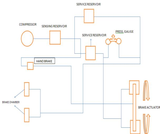
**Fig. 7.** The layout of Braking System set up.
