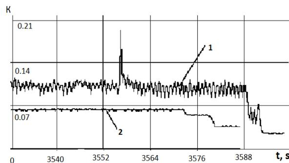
**Fig. 2.** Friction coefficient oscillograms: 1 – lubricant Soliton, 2 – lubricant Soliton with AWA.
