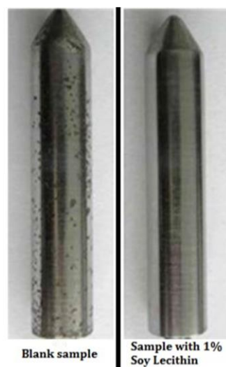
Fig. 5. Rods of Rust preventing characteristic test: Blank sample mineral base oils without Soy Lecithin shows a moderate rusting and blend contained 1 % of Soy Lecithin shows no rusting.
