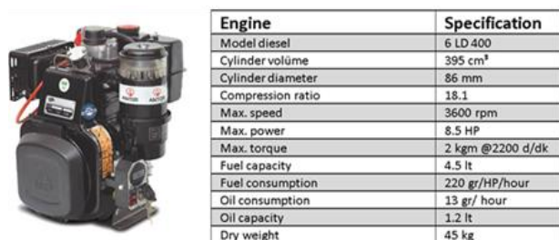
Fig. 1. Anadolu motor Antor 6 LD 400 diesel engine and its technical specifications.
