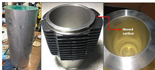
Fig. 3. Aluminum block drilled and honed as the same of Anadolu motor Antor 6 LD 400 diesel engine.
