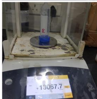
Case 3 Weight of falcon tube with wear particles
