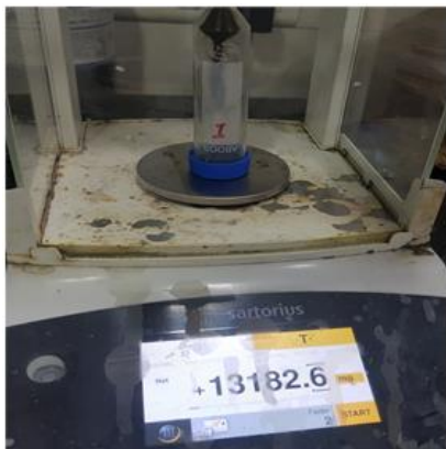
Case 3 Weight of falcon tube with wear particles
