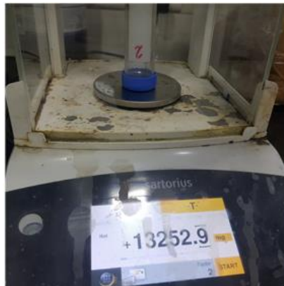
Case 3 Weight of falcon tube with wear particles
