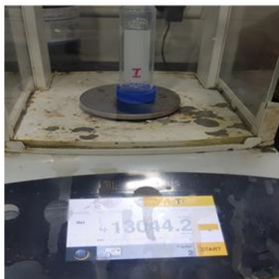
Case 3 Weight of falcon tube with wear particles
