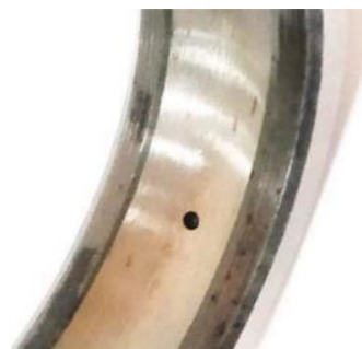
Fig. 3. Defect in outer race [8].
