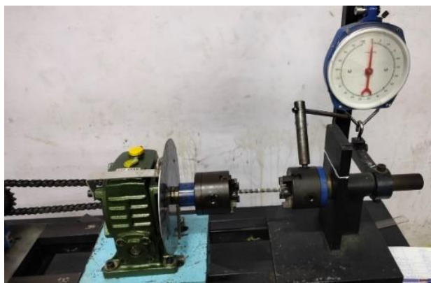
Fig. 13. Reduction gear loading in torque tests.
