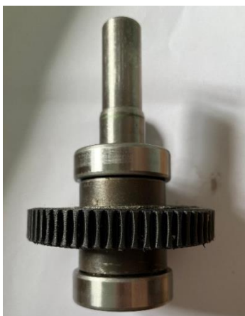
Fig. 12. Worm gear ring composite assembly.
