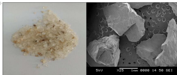
Fig. 3. Abrasive material and its morphology utilized in the current investigation.
