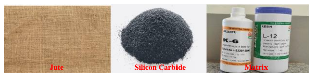
Fig. 1. Components employed in the creation of the intended composites.
