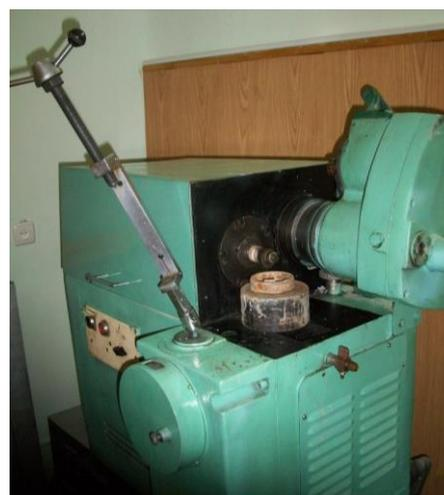
**Fig. 3.** General view of the SMC-2 friction machine.
