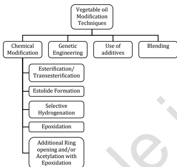
**Fig. 3.** Vegetable oil modification techniques to improve pour point and thermo-oxidative stability.
