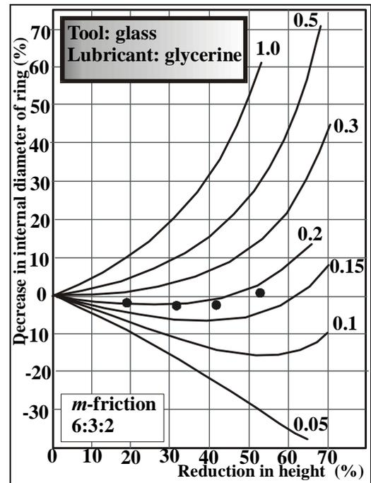
Figure 3. Experimental results, calibration curves Lee and Altan,  $m$ -friction
