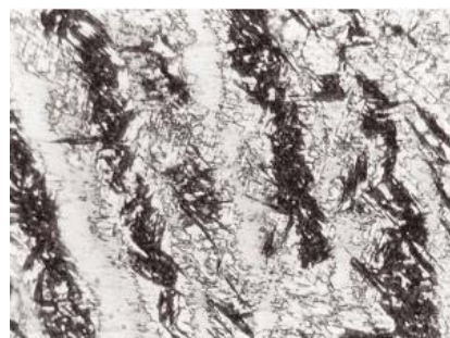
Figure 4: Microstructure of deposited layer for the second pass hardfacing (X 375)
