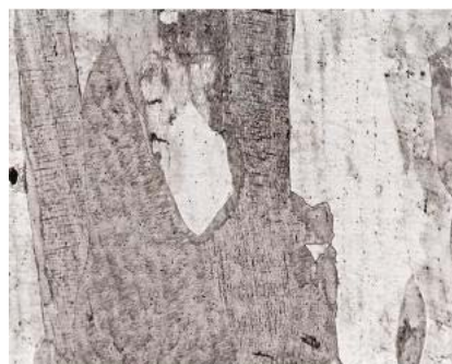
Figure 5: Microstructure of deposited layer for the third pass hardfacing (X 100)
