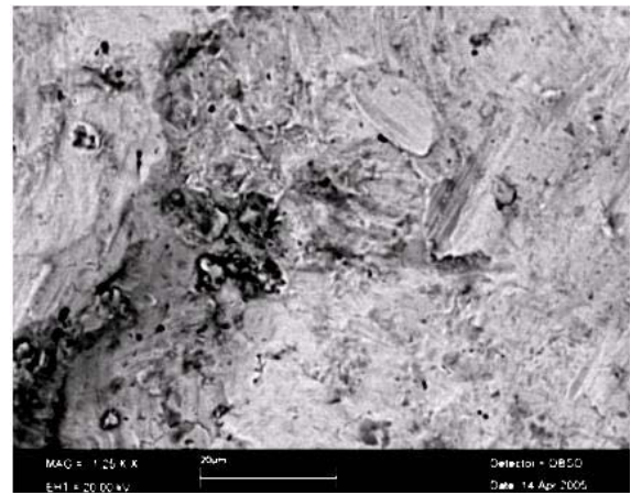
Figure 10: Top view of eroded surface the belonging of third layer deposited. (Impact angle: 30°)
