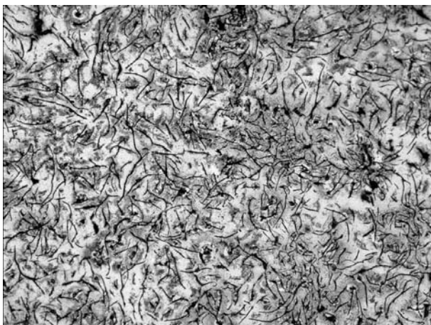
Fig. 2: Microstructure of GJL 215, X200, Nital attack
