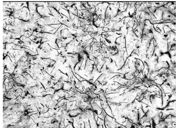
Fig. 3: Microstructure of GJL 155, X200, Nital attack
