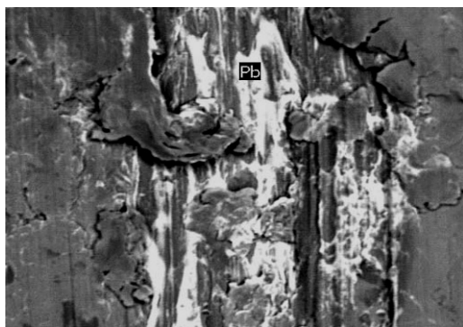
Figure 2. Micrograph of the friction surface of materials IPM under dry friction in vacuum /x 1000/.
