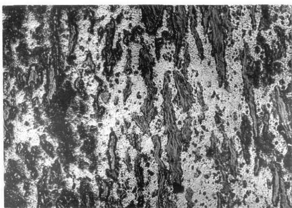
Figure 7. Micrograph of the structure of self-lubricating composite material IPM-306
