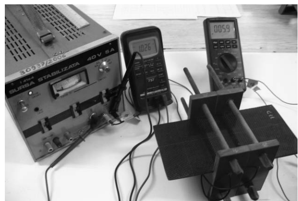
Figure 3. Experimental arrangement for longitudinal conductivity determination. Van der Pauw technique.
