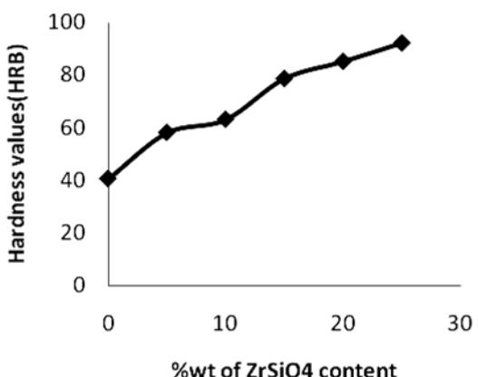
**Figure 9.** Variation of hardness with weight percentage of ZrSiO<sub>4</sub> content
