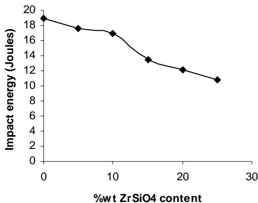
**Figure 11.** Variation of impact energy with weight percentage of ZrSiO<sub>4</sub> content
