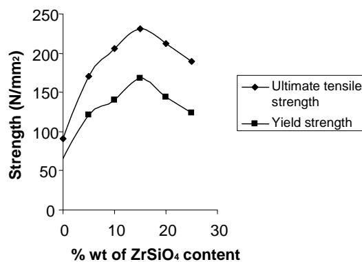
**Figure 10.** Variation of ultimate tensile and yield strength with weight percentage of ZrSiO<sub>4</sub> content
