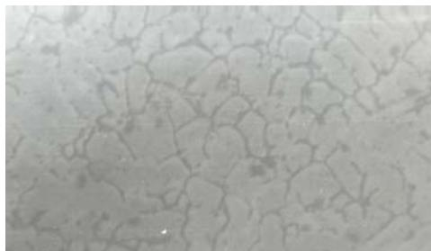
**Figure 4.** Microstructure of Al-4.5Cu alloy reinforced with 10%  $\text{ZrSiO}_4$ . More enlargements of the grain boundaries with larger patches of  $\text{ZrSiO}_4$  (black) magnification x 125
