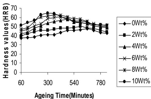
**Figure 2.** Variation of the Hardness values with Ageing Time at Ageing Temperature of 200°C
