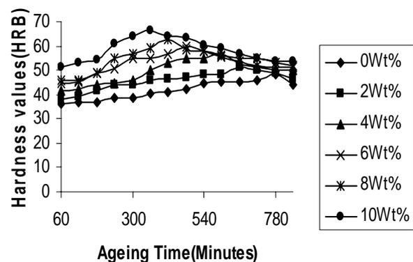
**Figure 1.** Variation of the Hardness values with Ageing Time at Ageing Temperature of 100°C
