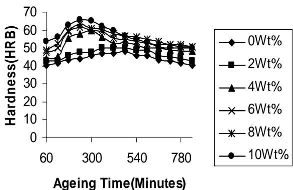
**Figure 3.** Variation of the Hardness values with Ageing Time at Ageing Temperature of 300°C
