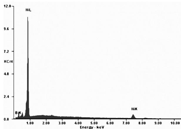
**Figure 6.** EDX spectra of Ni-B coating
