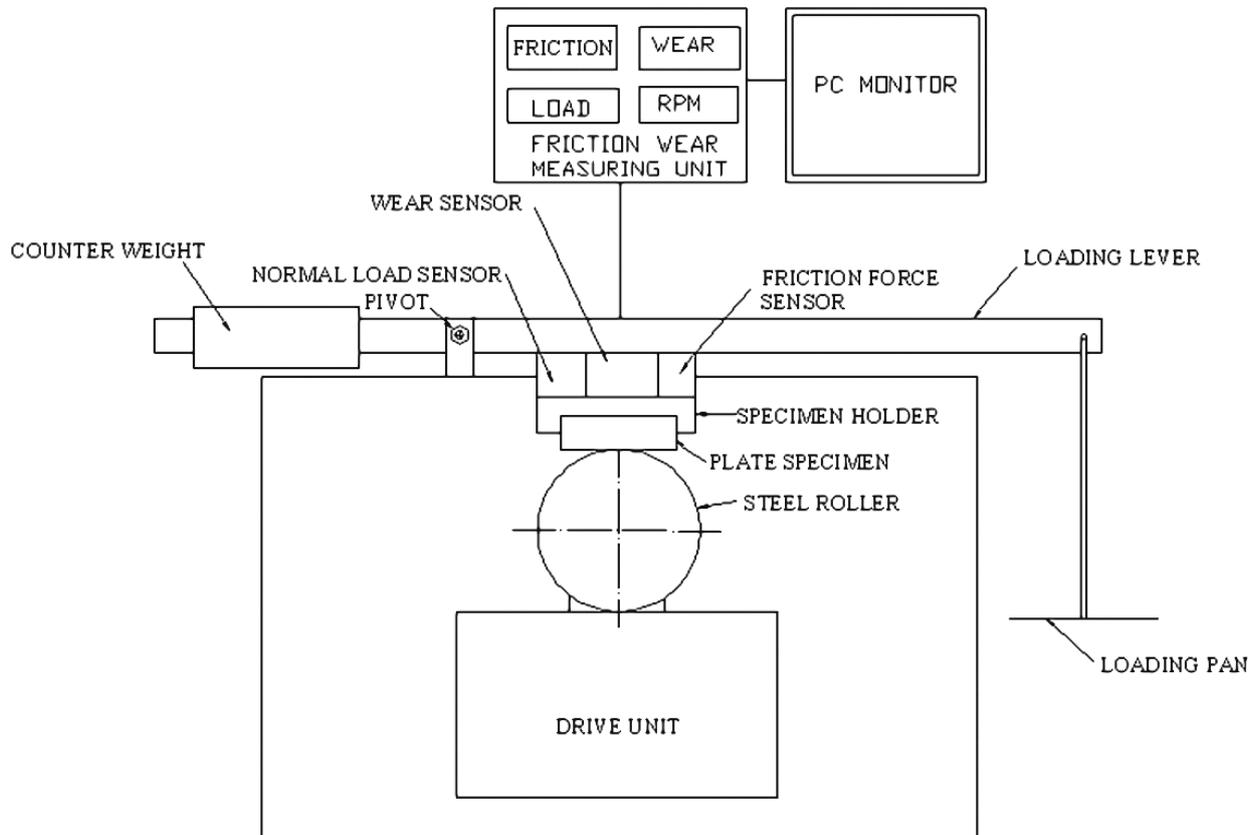
**Figure 3.** Schematic diagram of the multi-tribotester
