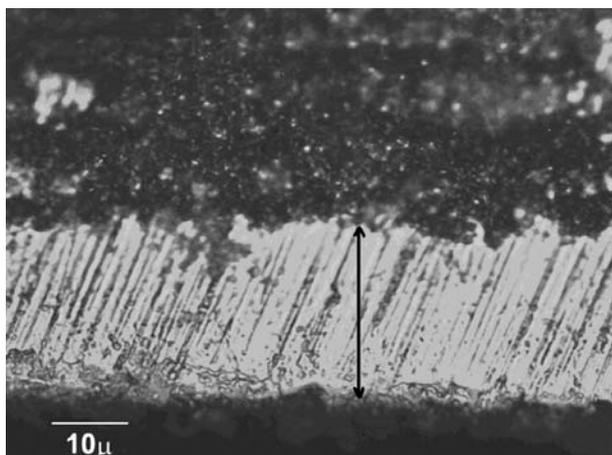
**Figure 2.** Optical micrograph of Ni-B coating cross-section
