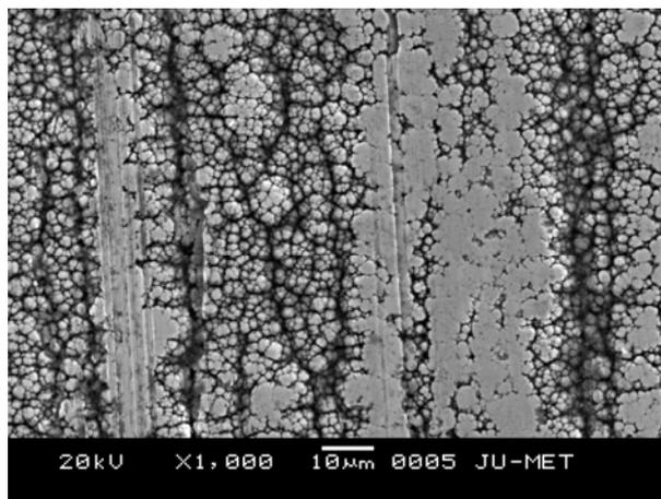
**Figure 9.** SEM picture of coating surface after friction testing
