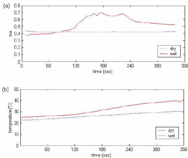
**Figure 9.** Results of the lining friction test at wet and dry conditions: (a) coefficient of friction, (b) temperature
