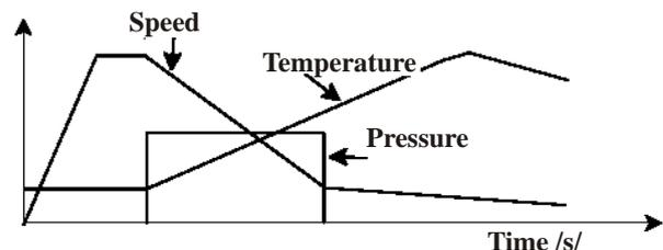
**Figure 10.** Variations of characteristic values during cold brake tests
