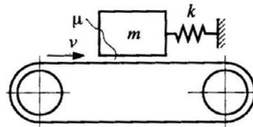
**Figure 4.** Negative  $\mu$ -velocity slope model
