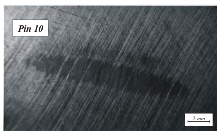
c) Pins No. 9 and 10 – lubricant with 6% MoS 2 - B.M. - Č5742 and Č4751
