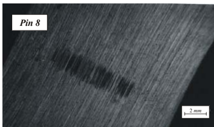
b) Pins No. 6 and 8 - lubricant with 6% MoS 2 – F.M. - UTOP 55
