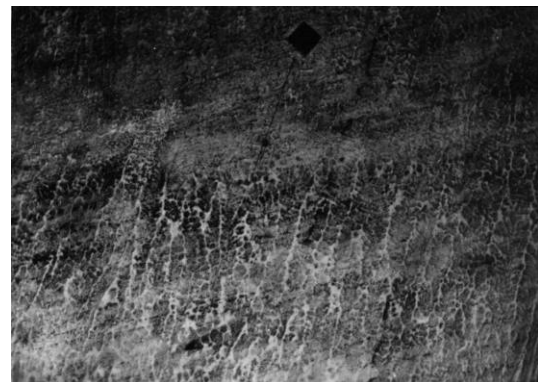
F. M. UTOP 55 - Hard-faced layer HV1= 700 Dendrite structure directed perpendicularly to the hard-faced metal surface
