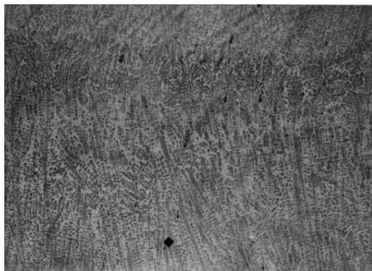
F. M. UTOP 38 – Hard-faced layer HV1= 580 Dendrite structure directed perpendicularly to the hard-faced metal surface
