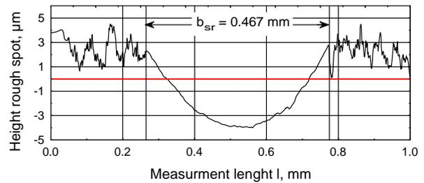
**Figure 13.** Layout of the wear scare - block No 1 (after the contact of 60 min)
