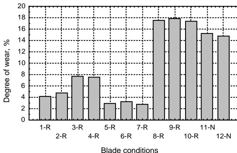
1-R and 2-R – ABRADUR 58; 3-R and 4-R – CrWC 600; 5-R, 6-R and 7-R – E DUR 600; 8-R, 9-R and 10-R – E Mn17Cr13; 11-N and 12-N – NEW BLADES (B. M.)
