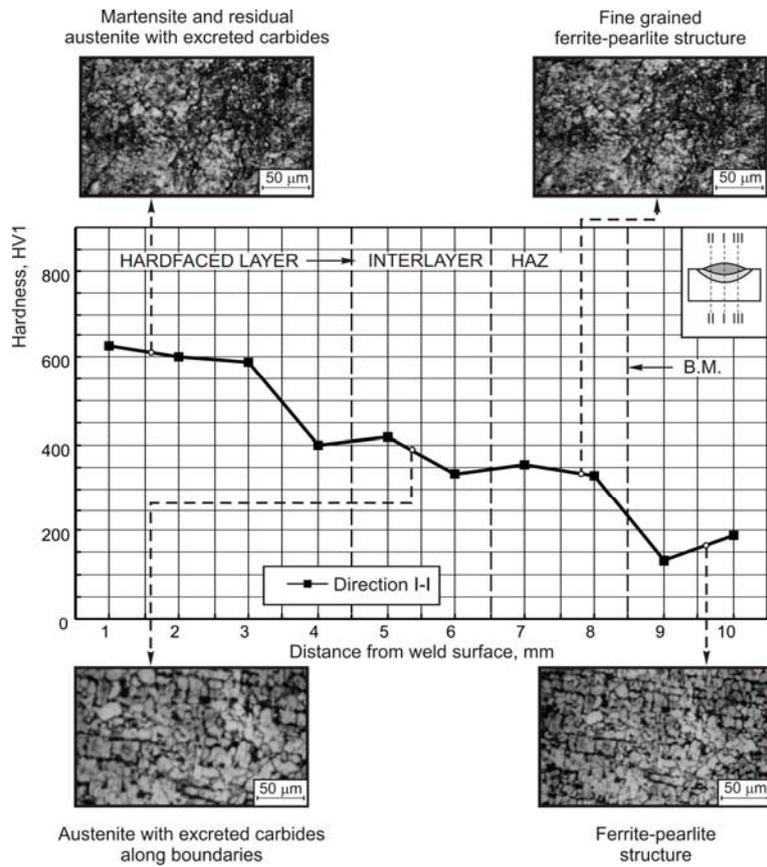
**Figure 4.** Microstructure of the hard faced metal zones: B.M. - Č0361, interlayer - INOX B 18/8/6 and hard faced layer - E DUR 600
