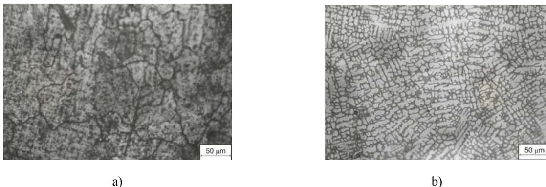
**Figure 7.** Microstructure of the hard faced layer: (a) E Mn17Cr13 and (b) INOX B 18/8/6
