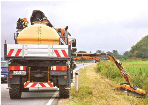
**Figure 1.** Machine and device for vegetation maintenance and grass cutting
