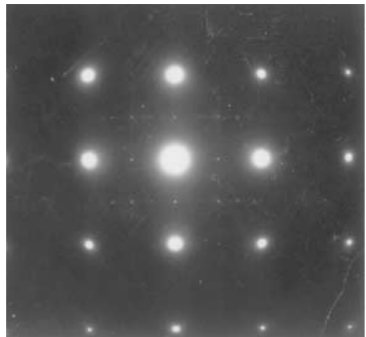
Micrograph 6. TEM/ SADP showing S' precipitates in the composite over-aged
