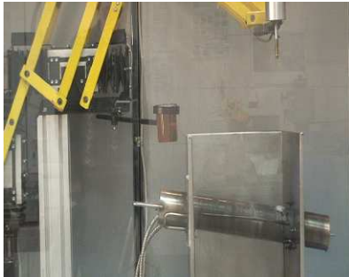
Figure 5. Consecutive images from the film recorded for the fluid HFC Prista, tested at 700°C
