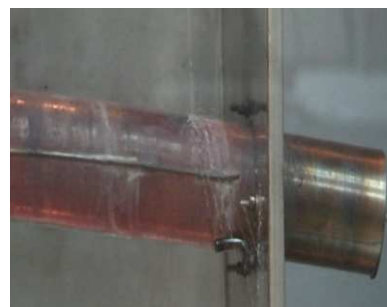
Figure 7. Images from the film recorded for the mineral oil MHE 40 Prista, tested at 460°C
