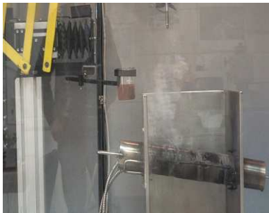
Figure 6. Three images from the film recorded for the mineral oil MHE 40 Prista tested at 450°C
