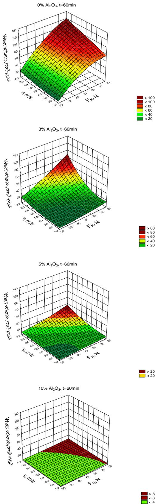
**Figure 8.** Relationships between wear scar width and normal load and sliding speed, for different mass weight of the reinforcements
