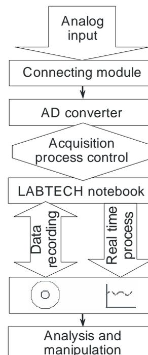
Figure 3. Block diagram of data acquisition process
