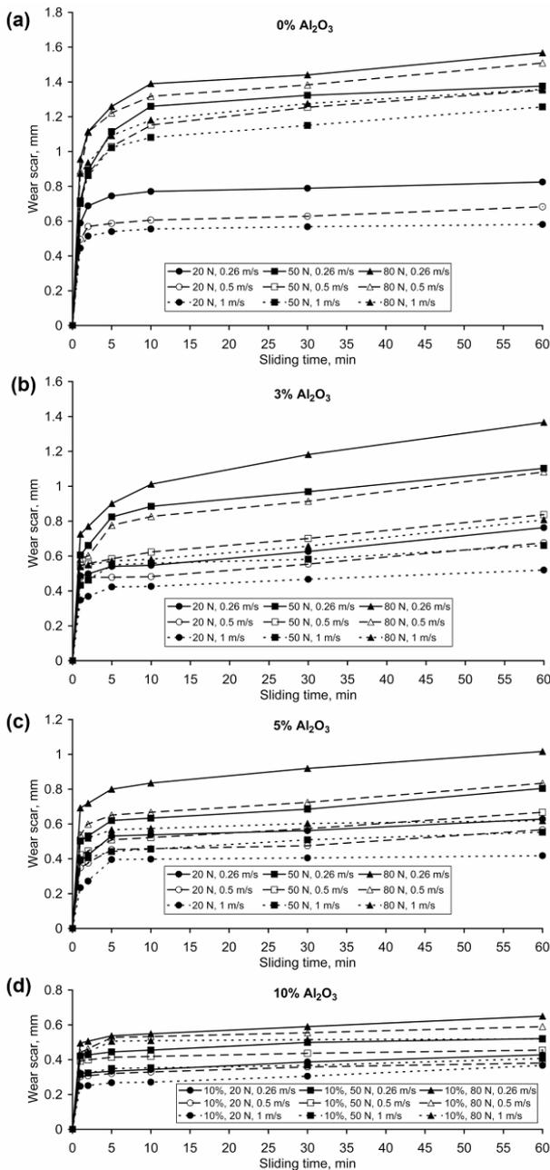
**Figure 6.** Wear curves of: (a) ZA-27 matrix alloy, (b) MMC 3% Al<sub>2</sub>O<sub>3</sub> (c) MMC 5% Al<sub>2</sub>O<sub>3</sub> (d) MMC 10% Al<sub>2</sub>O<sub>3</sub>
