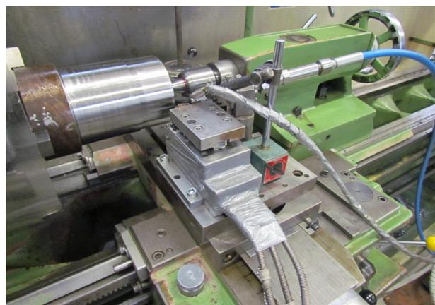
Fig. 4. Experimental setup on machine.
