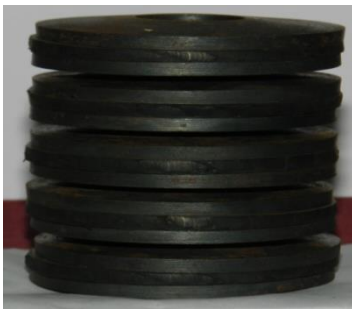
Fig. 5. Series combination of 'EPDM-EN 45' disc spring.
