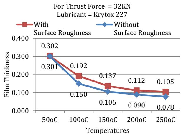
Fig. 9. Effect of surface roughness at 32KN Force for Krytox 227.
