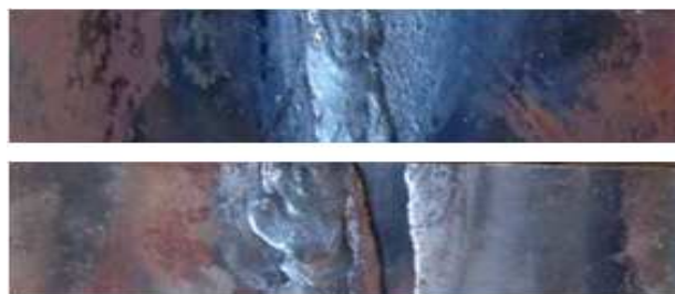
Fig. 3. Typical highlighted Zn-Mn-Ag brazed and tensile tested joint.
