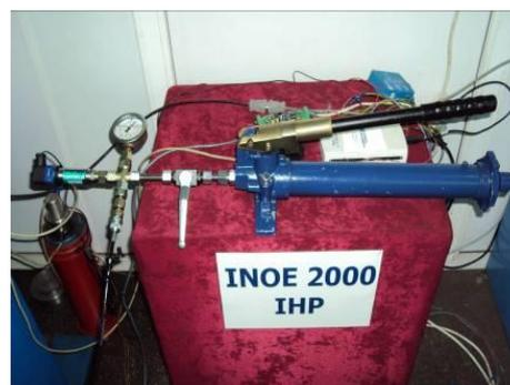
Fig. 9. The hand oil pump
