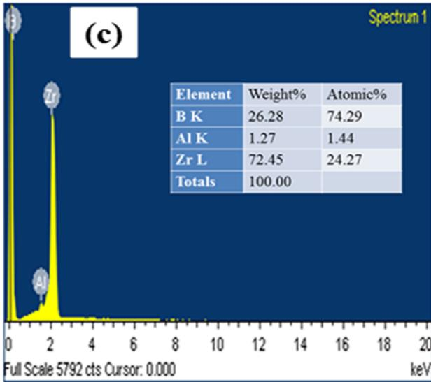
Fig. 5. (a) and (b) Morphology of ZrB<sub>2</sub>particle at higher magnification (c) EDS spectrum of ZrB<sub>2</sub>.
