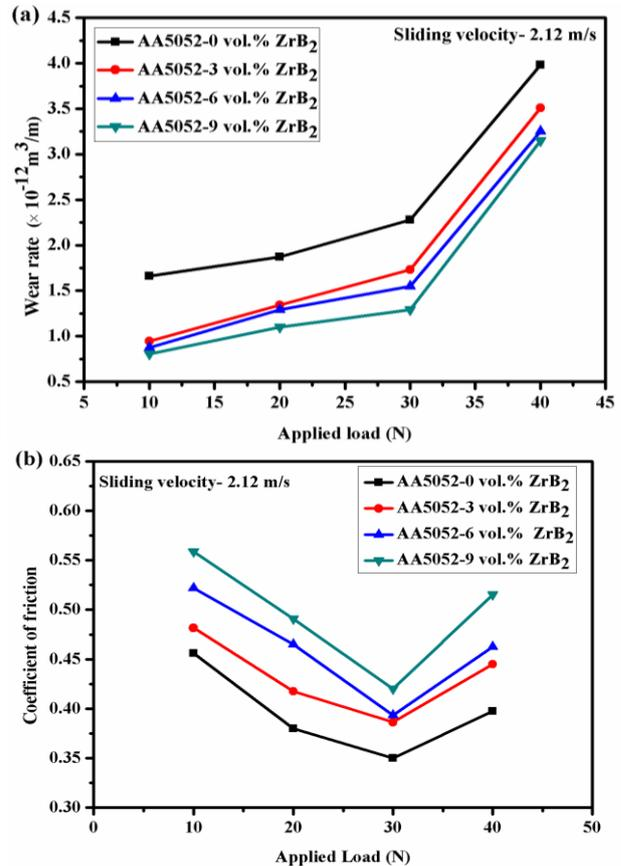
**Fig. 11.** (a) Variation of wear rate with applied load and (b) Variation of COF with applied load.
