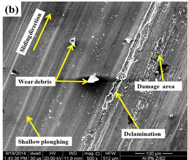
Fig. 15. Wear surface morphology of (a) AA5052 alloy (b) 9 vol.% ZrB<sub>2</sub> composite at 20 N load and 2.12 m/s sliding velocity.
