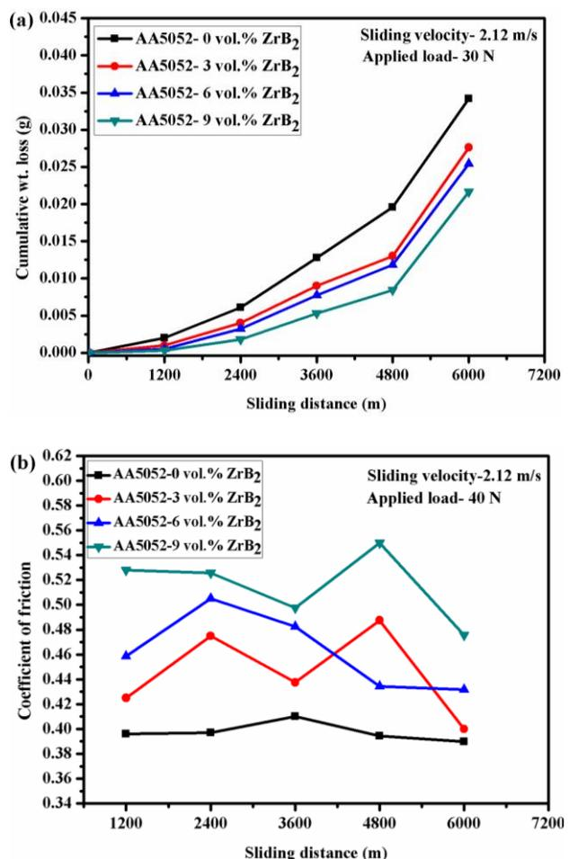
Fig. 9. Variation of (a) cumulative wt. loss and (b) COF with sliding distance.
