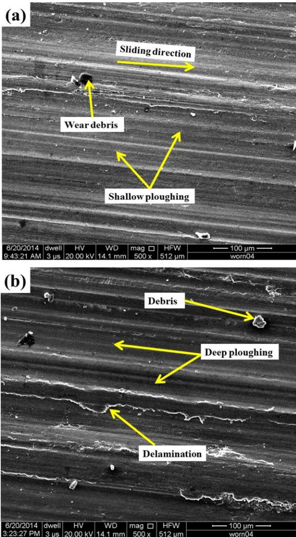
**Fig. 10.** Wear surface morphology of 6 vol.% ZrB<sub>2</sub> composite at 30 N load and 2.12 m/s sliding velocity after sliding distance of (a) 1200 m (b) 6000m.
