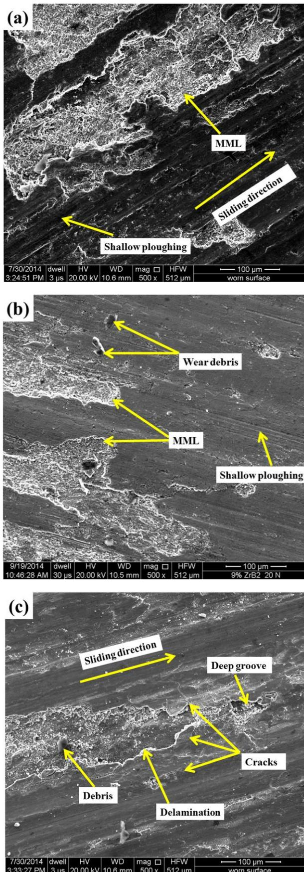
**Fig. 12.** SEM micrographs of wear tracks at different loads for composite with 9 vol.% ZrB<sub>2</sub> particles at 2.12 m/s sliding velocity (a) 10 N, (b) 20 N and (c) 40 N.
