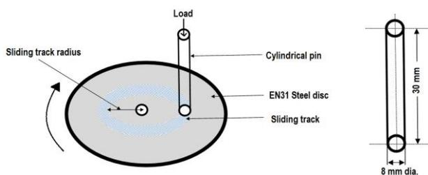
Fig. 1. Schematic diagram of pin-on-disc apparatus.
