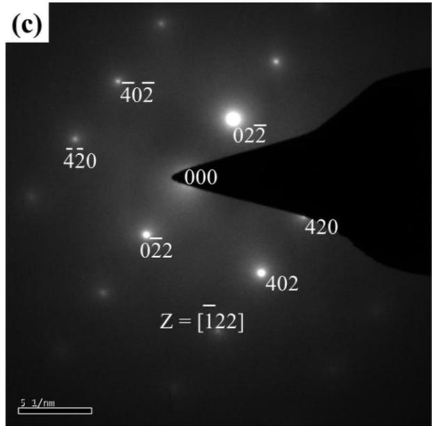
Fig. 6. TEM micrographs of (a) rectangular morphology (b) SAD pattern of ZrB<sub>2</sub> and (c) SAD pattern of matrix.
