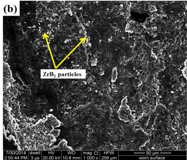
Fig. 14. SEM micrographs of wear tracks of composites with different % ZrB<sub>2</sub> particles at 30 N load and 2.12 m/s sliding velocity showing larger number of particles in MML (a) 3 vol.% and (b) 9 vol.%.
