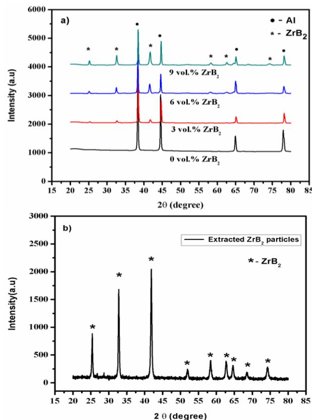
Fig. 2. XRD pattern of (a) Prepared in-situ composites (b) Extracted  $ZrB_2$  particles.
