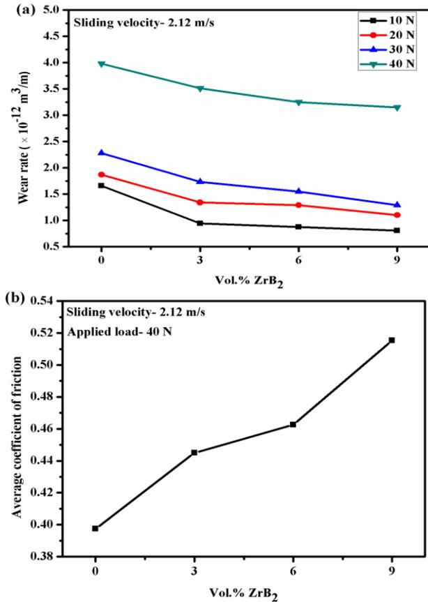
Fig. 13. Variation of (a) wear rate with vol.% ZrB<sub>2</sub> (b) COF with vol.% ZrB<sub>2</sub>.
