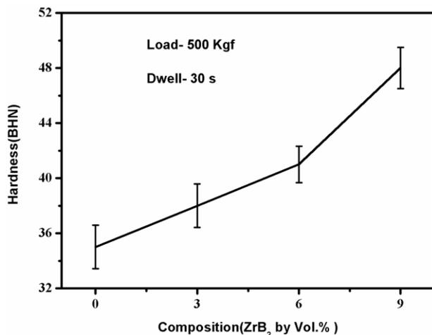
Fig. 8. Variation of hardness with vol.% of ZrB<sub>2</sub>.
