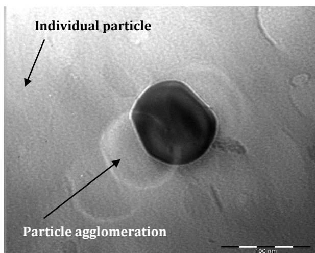
**Fig. 6.** TEM image of UCSNPs obtained at 70 hours milling and 5 CR.
