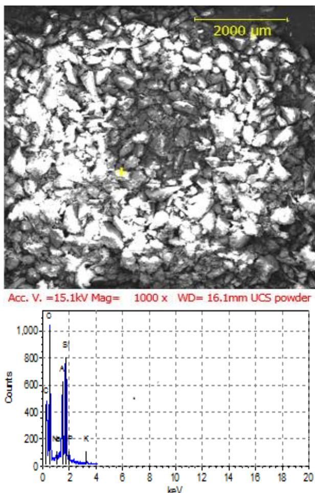
**Fig. 3.** SEM micrograph/EDS spectrograph of the UCS powder.
