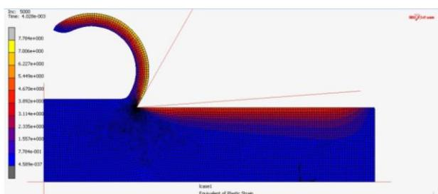
Fig. 3. Chip morphology and plastic strain.
