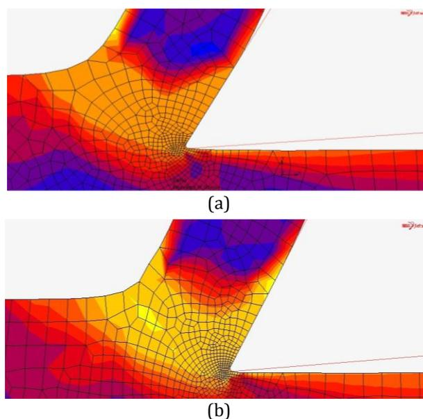
Fig. 5. Stresses in the primary and secondary deformation zone when (a) Coulomb ( $\mu=0.4$ ) and (b) stick-slip ( $m=0.4$ ) model is considered.
