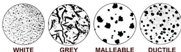
Fig. 1. Example of microstructures.
