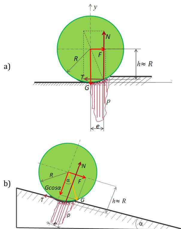
Fig. 1. The equilibrium of the body in movement of rolling.
