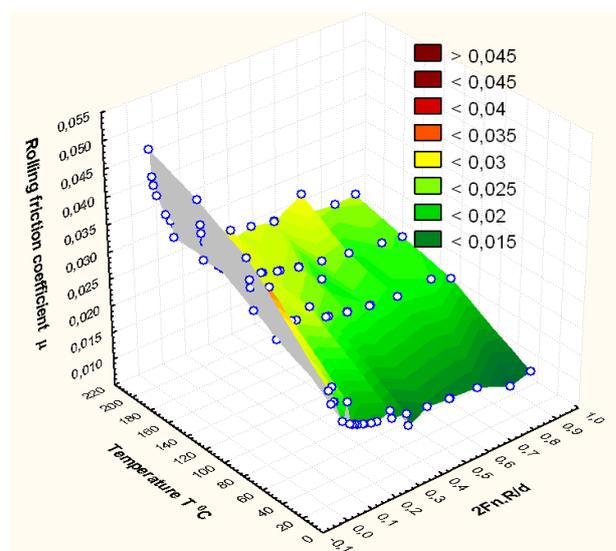
Fig. 6. 3D preview experimentally obtained depending coefficient of friction on the temperature and contact geometry.
