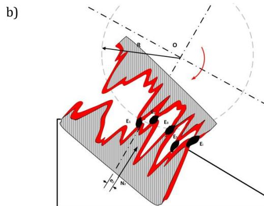
**Fig. 3.** Position of resultant force N without heating of the contact pair (Fig. 3a.), and with heating the contact pair (Fig. 3b.).
