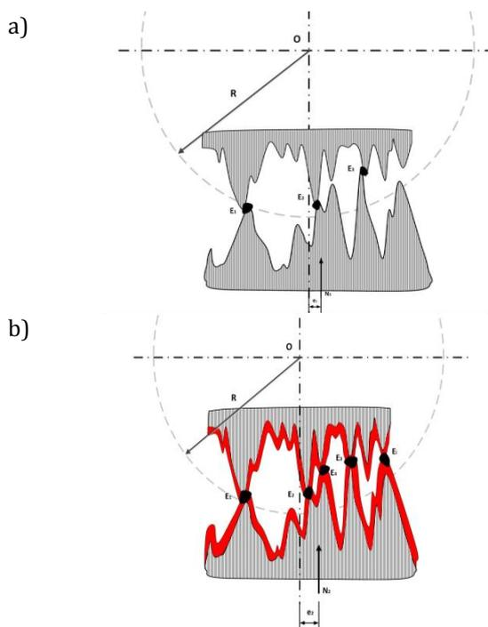
**Fig. 2.** The real contact area of sphere and flat surface before heating (Fig. 2a.), and after heating (Fig. 2b.).
