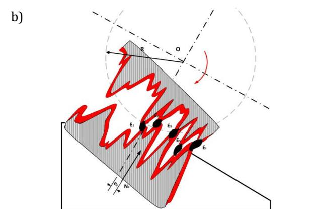
**Fig. 3.** Position of resultant force N without heating of the contact pair (Fig. 3a.), and with heating the contact pair (Fig. 3b.).
