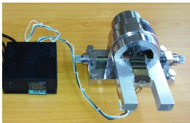
Fig. 4. Photographic representations of tribometer.
