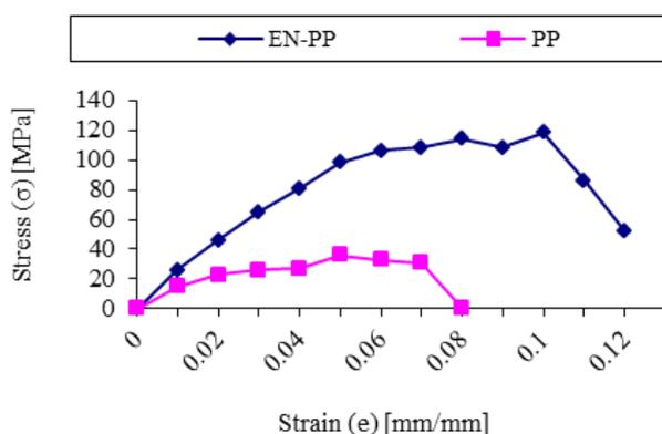
Fig. 12. Strength test of EN-PP and PP.
