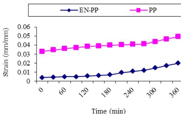
Fig. 13. Creep test of EN-PP and PP under 5 kg load.
