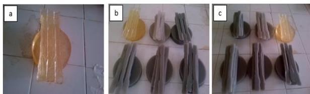
**Fig. 2.** Photographic representations of (a) NE test samples (b) 75 µm series EMSB test samples (c) <75 µm series EMSB test samples.
