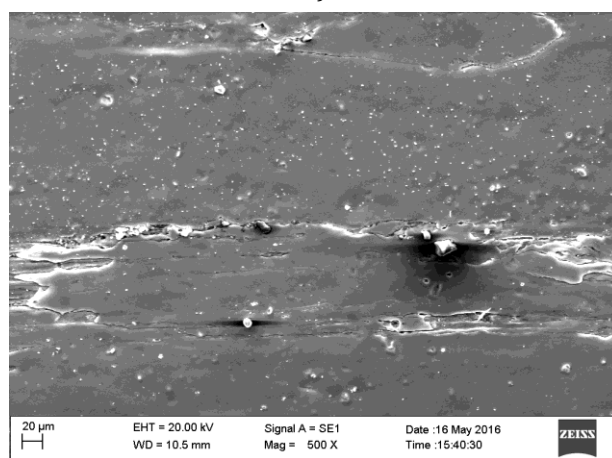
Fig. 5. SEM of the longitudinal section of the unextruded billet after extrusion with implanted electroless nickel plated micro SiCp.
