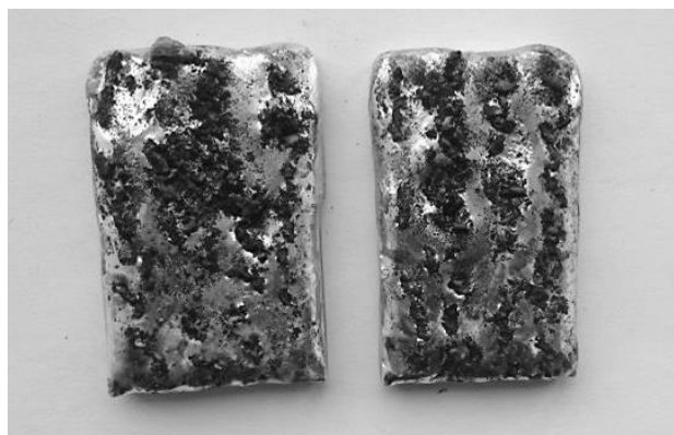
a) Specimens welded without flux
