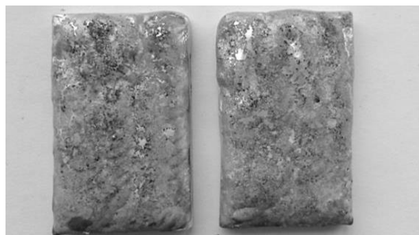
b) Specimens welded with flux coated particles
