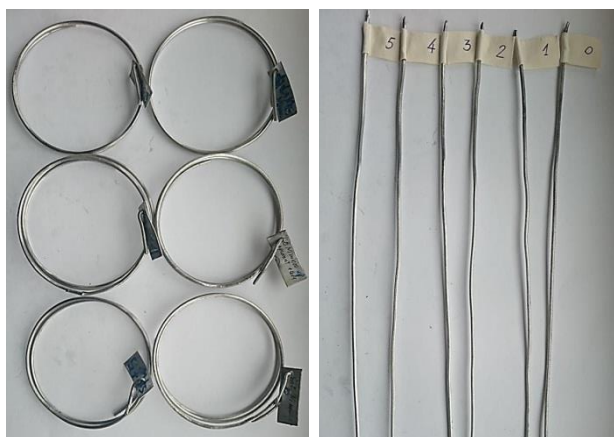
Fig. 4. Pictures of the obtained through extrusion additive material (wire filler).
