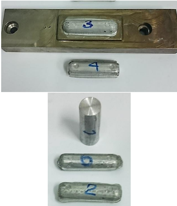
Fig. 1. Forged samples obtained at subsequent positioning - number of strokes after 900 rotation by impression-die forging.
