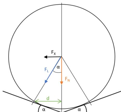
**Fig 6.** Ball-on-plate friction measurement function principle (adopted from [18]).
