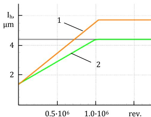
**Fig. 3.** The dependence of wear (the convergence of surfaces) for the 2nd (curve 2) and 3rd (curve 1) main bearings on rev.
