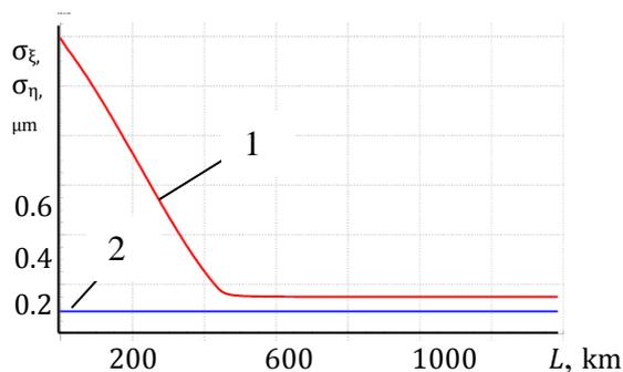
**Fig. 2.** The heights of surface roughness of bearing (1) and shaft (2) in function of friction distance.
