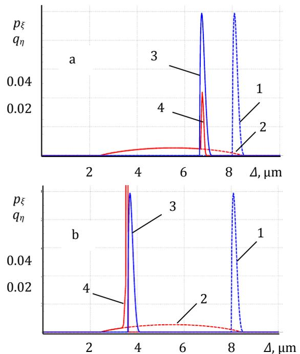
**Fig. 1.** The distribution of the heights of roughness of contact surfaces: after run-in time (a) and after friction distance 1380 km (b): 1, 2 - initial curves for shaft and bearing respectively; 3,4 - curves after interaction.
