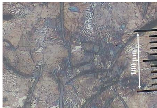
Fig. 5. Microstructure of C-MBB showing ferrite, pearlite and flake graphite phase.
