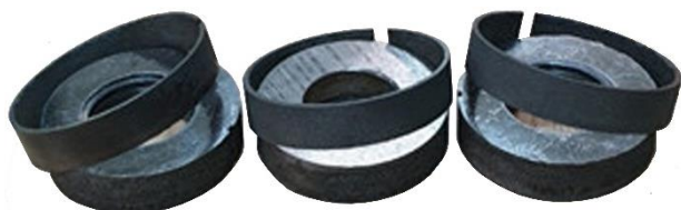
Fig. 5. Coating separated from the base steel
