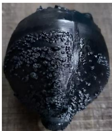
Fig. 11. Bubble formation due to a small porosity in the printed part .
