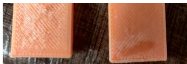
Fig. 10. PLA with THF solution optimised result.
