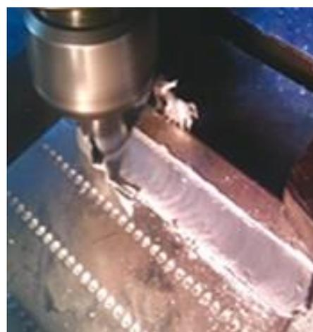
**Fig. 1.** Specimen during friction stir process.
