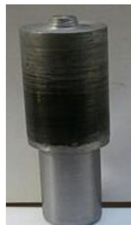
**Fig. 2.** Shoulder with threaded pin.
