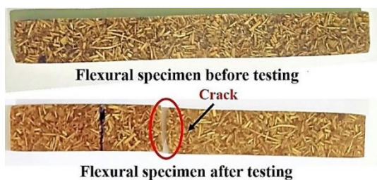
Fig. 4. Before and after test image of flexural specimen.
