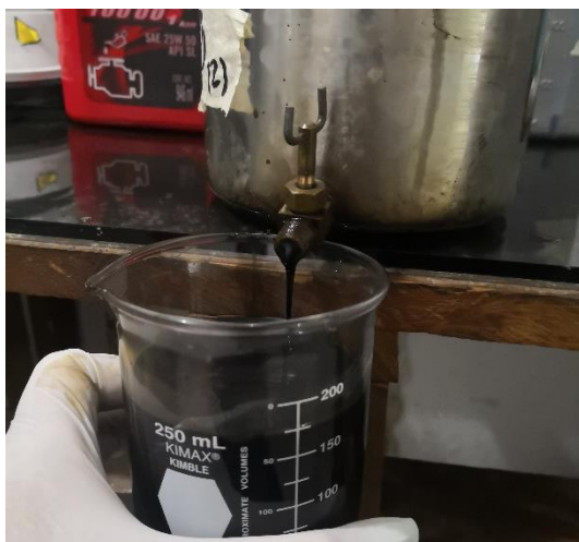
Fig. 1. ULO leachates, after the application of sulfuric acid and nonylphenol.
