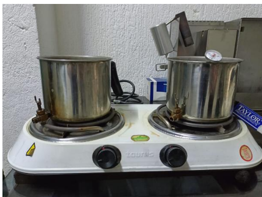
Fig. 2. Stove with knobs to regulate the proposed temperatures with a 250 C mercury thermometer.
